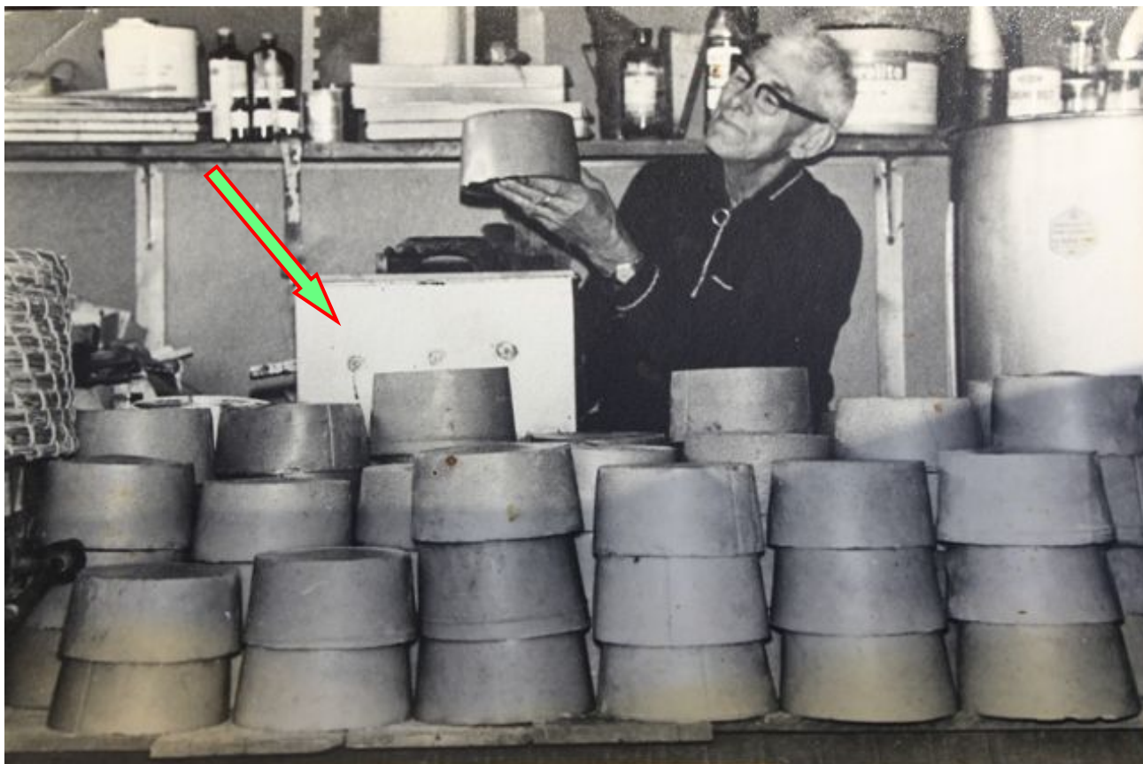
Figure 5. George Wakeford with a crop of beeswax rendered from cappings. Note the Wakeford Wax Extractor (arrowed) in the centre. I believe this to be the second prototype, not the final version. He ran the molten wax (from the spout seen on the left) into tapered tins (one just seen under the spout) obtained from the butcher that had previously contained lamb's liver from New Zealand. This photograph was probably taken in the shed of Tom Haffenden, who worked closely with George and at one stage was the WGBKA Treasurer.
